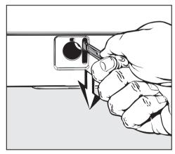
■ Use a spoon handle or similar to pull the emergency door latch downwards (see illustration). The drum door will open.
